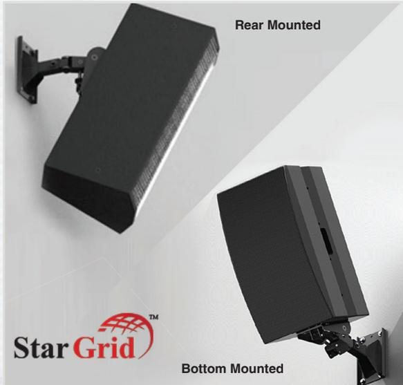
The MM-120 Speaker Mount supports speakers from its back and bottom or top panel, weighing up to 120 lb., and is fully adjustable in both pan and tilt aiming, plus comes with a telescoping wall arm to adjust the relative distance between the speaker and the wall.
