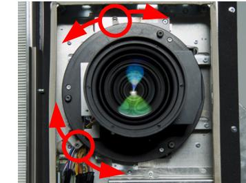
7 Using the tabs, rotate the shift plate until an optimum center focus is achieved.
