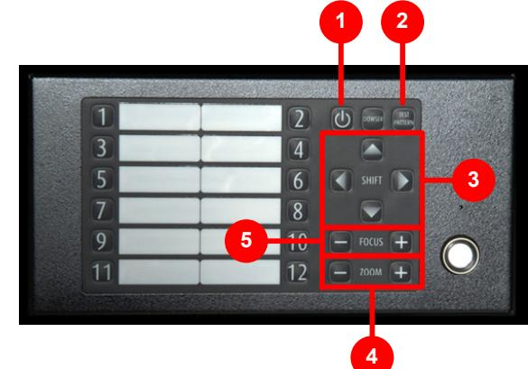
Align the image to fill the screen masking using the following functions:
