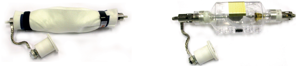
Image 4-1: Left: Xenon lamp wrapped in a protective cloth. Right: Xenon lamp captured in a protective container.
