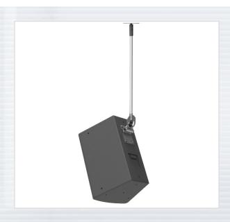
The MM-3RDX-18 is an adjustable ceiling speaker mount that provides pan, tilt & roll adjustments. It supports and aims speakers that are equipped with either the 2 X4-1/4 or the 2-3/4" X 5" 4-point mounting pattern.
