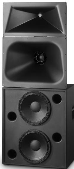
Developed specifically for the unique requirements of professional motion picture playback, the SC-423C extends QSC's commitment to the cinema market. As a member of the DCS Digital Cinema Speaker Series, the SC-423C is a 3-way, selectable bi or tri-amplified screen channel loudspeaker system comprised of two main units—the MH-1075C mid-high frequency system and the LF-4215 low-frequency system.
