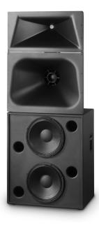
Developed specifically for the unique requirements of professional motion picture playback, the SC-423C extends QSC's commitment to the cinema market. As a member of the DCS Digital Cinema Speaker Series, the SC-423C is a 3-way, selectable bi or tri-amplified screen channel loudspeaker system comprised of two main units—the MH-1075C mid-high frequency system and the LF-4215 low-frequency system.
