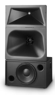
Developed specifically for the unique requirements of professional motion picture playback, the SC-414 extends QSC's commitment to the cinema market. As a member of the DCS Digital Cinema Speaker Series, the SC-414 is a 4-way, selectable tri or quad-amplified screen channel loudspeaker system comprised of two main units — the MHV-1090 mid-high-very high-frequency system and the LF-4115 low-frequency system.
