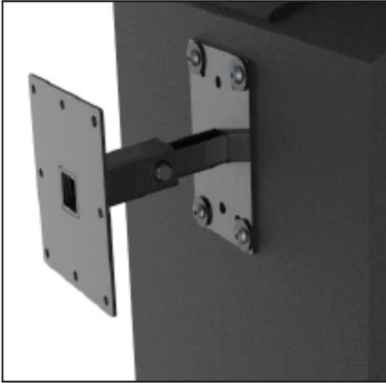
The WM-0-15-60 wall mount is an excellent choice for various wall mounting positions as well as 0° and 15° speaker tilt angles. The speaker are secured to standard loud speaker mounting hole patterns, 5"x2.75" and 4" x 2.25" located on the rear of the speaker cabinets. This mount secures to speakers by way of standard 4 hole mounting pattern including 5" X 2 3/4 and 4 X 2 1/4 located on the rear panel of speaker cabinet.
