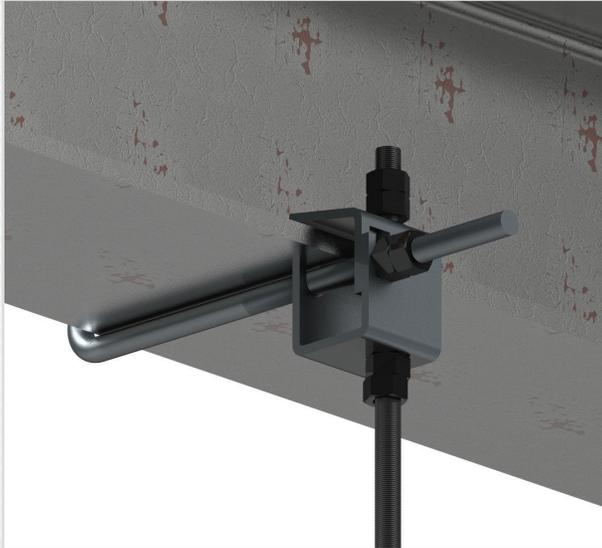
Standard, pre-engineered channel style beam clamps anchor to a building's structure and offer a safe and predictable method of rigging grids and other objects from overhead. This hook style beam clamp is adjustable and mounts flush underneath the building's I-Beam's flange. Use the BC-2824-series hook style beam clamp to provide a load rated overhead rigging point from structural I-Beams with widths ranging between 2" and 6", 6" and 9" or 9" and 12".
