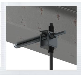
Standard, pre-engineered channel style beam clamps anchor to a building's structure and offer a safe and predictable method of rigging grids and other objects from overhead. This hook style beam clamp is adjustable and mounts flush underneath the building's I-Beam's flange. Use the BC-2824-series hook style beam clamp to provide a load rated overhead rigging point from structural I-Beams with widths ranging between 2" and 6", 6" and 9" or 9" and 12".
